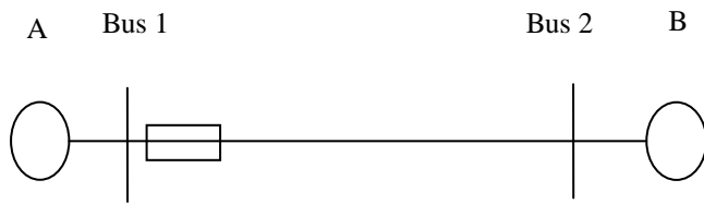
Fig. 2. Single line diagram of the power system
